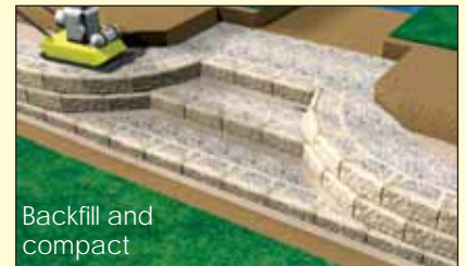
Install wall out from stairs
